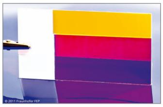
Dichroic filters, as used for example in cameras, can be manufactured with greater processing reliability using the new measuring technology. | © Fraunhofer FEP
