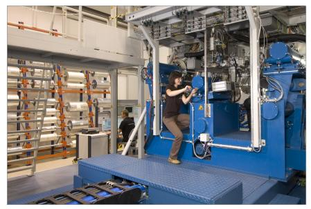
Pilot plant for the vacuum coating of plastic film in roll-to-roll mode. Existing processing lines such as these or industrial facilities can be refitted for the innovative process. © Fraunhofer FEP | Picture in printable resolution: www.fep.fraunhofer.de/press
