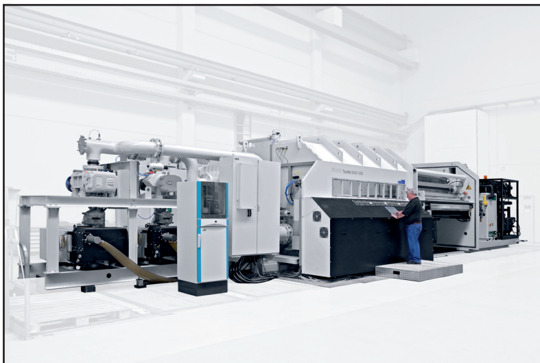
An industrial vacuum roll coater: »Applied TopMet Clear 2450« © Applied Materials, Inc.
