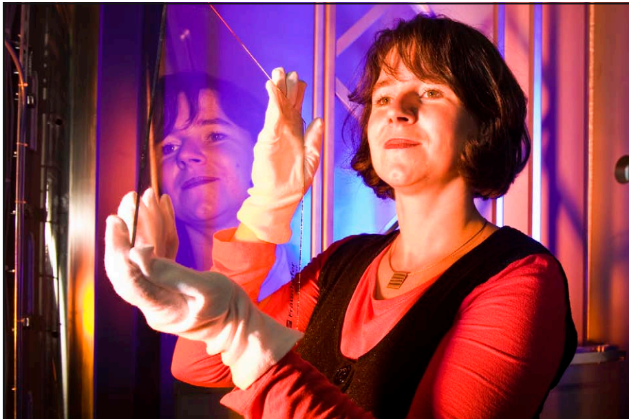
Glass plate with a transparent conducting layer based on titanium dioxide. The electrode material of the future? © Fraunhofer FEP
