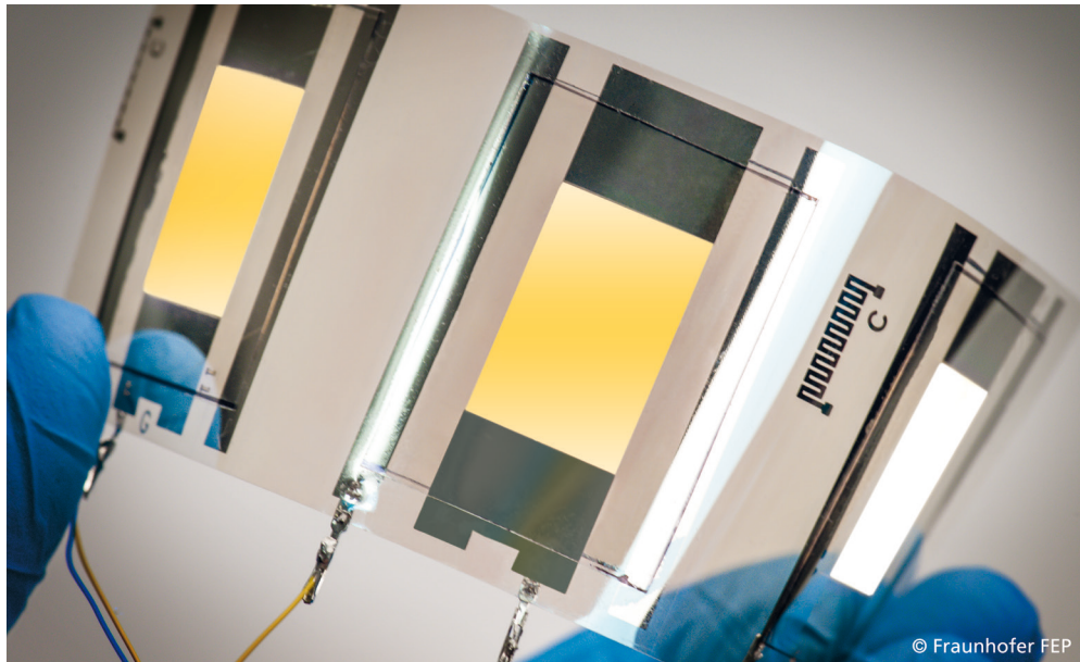
Flexible OLED of Fraunhofer COMEDD, built upon and encapsulated with functional films of Fraunhofer POLO
