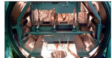
Fig. 2: CSS equipment for CdTe deposition
