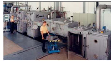
Figure 6: "MAXI" inline high-rate coating equipment at Fraunhofer FEP Dresden
