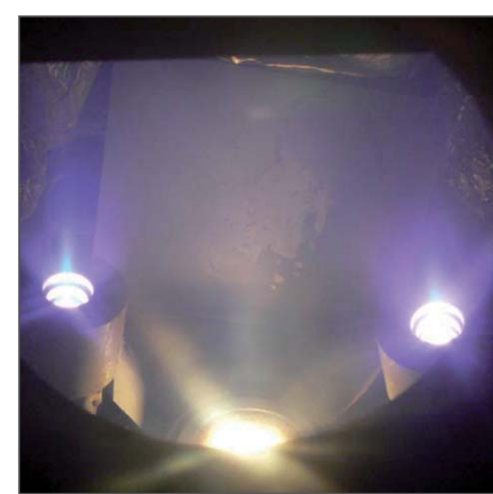
Figure 5: HAD process in action (crucible in the center, hollow cathodes at left and right side).
