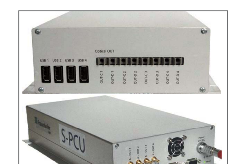
Figure 16: Spectrometric Process Control Unit - S-PCU (front and rear view)
