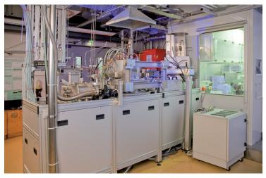
Fraunhofer researchers are using this lab coater to produce piezoelectric AIN layers for low power sensors in an economically feasible manner. © Fraunhofer FEP | Picture in printable resolution: www.fep.fraunhofer.de/press
