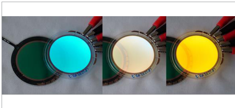
2-color variable transparent OLED module with activated blue, blue and yellow as well as yellow unit
