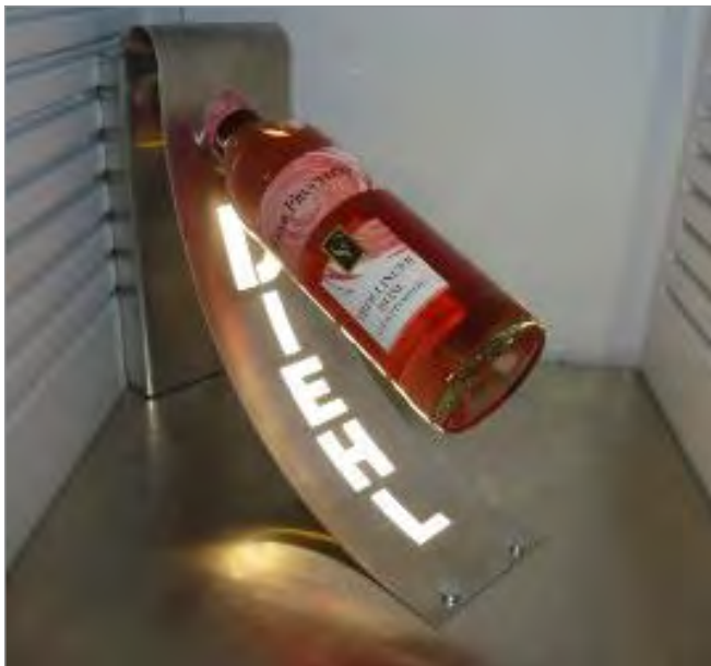
“Coolfood” OLED demonstrator from DIEHL using an OLED module fabricated by Fraunhofer FEP on flexible ultra-thin glass.
