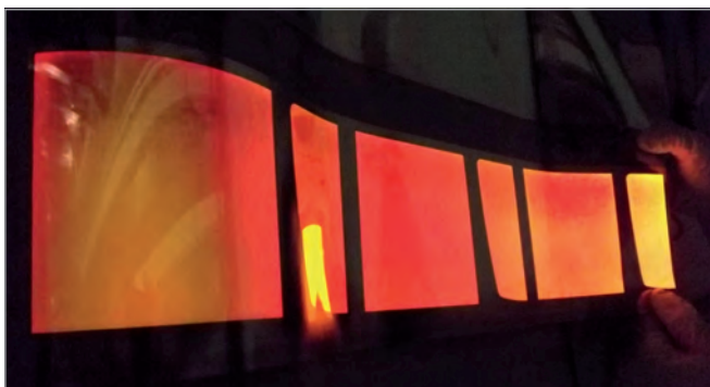
Flexible OLEDs produced at Fraunhofer FEP using roll-to-roll processing
