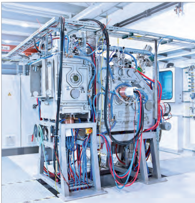
NOVELLA – facility for coating 3D components
