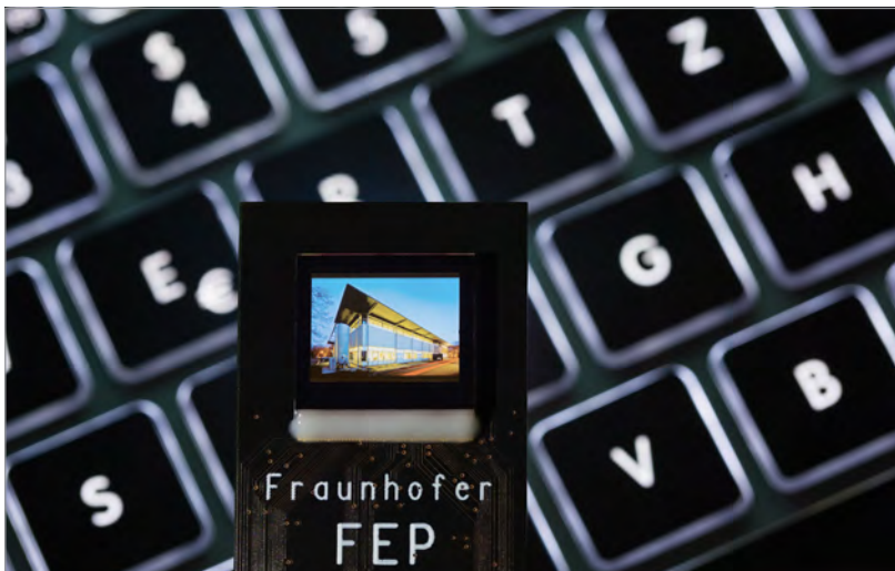
Bi-directional OLED microdisplay with embedded image sensor function
