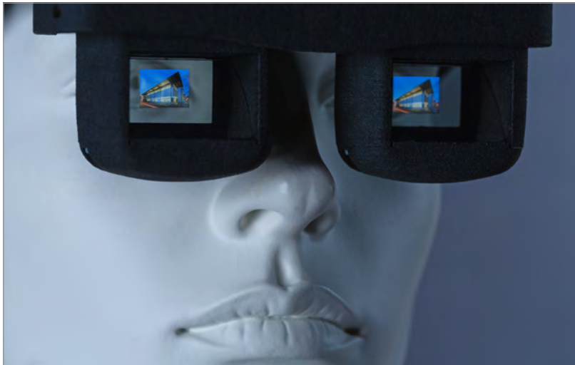
Interactive smart eye-glasses using bi-directional OLED microdisplays
