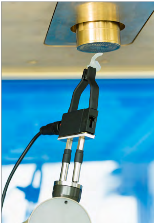
Electron exit window of the miniaturized electron beam source and robotic handling for applying electron beams to 3-D objects.
