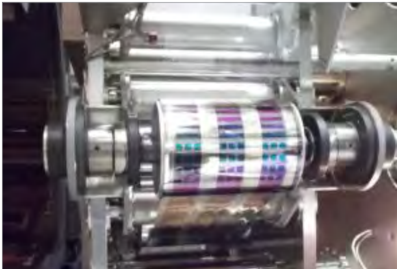
Detail of the Roll-to-Roll vacuum coater at Fraunhofer FEP
