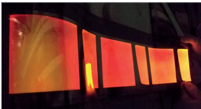
Photo 2: Flexible OLEDs produced at Fraunhofer FEP using roll-to-roll processing
