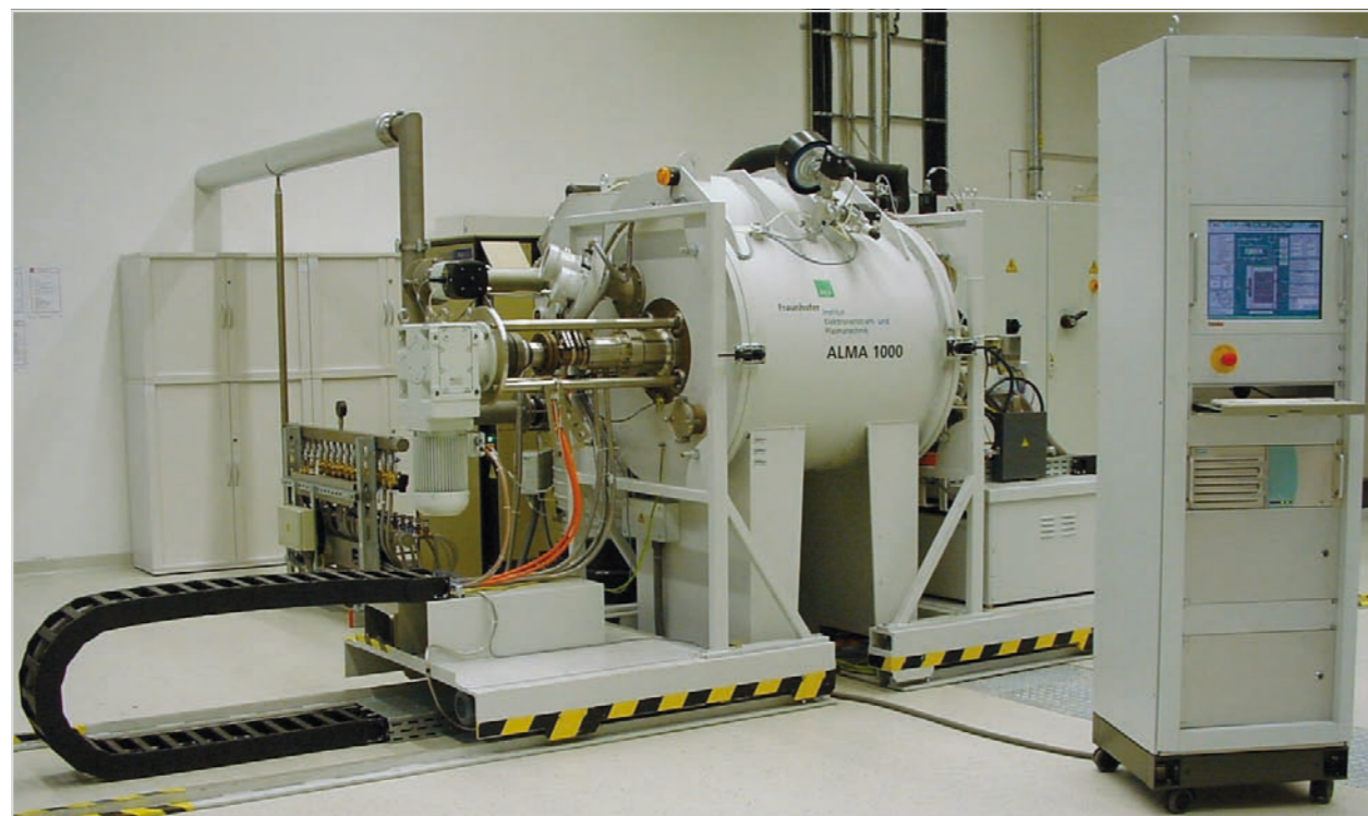
Fig. 1: The ALMA 1000 experimental plant for coating mass-produced products.
