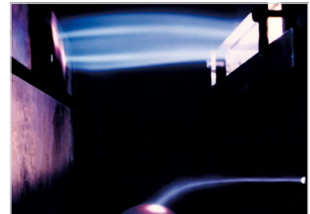
Fig. 2: Electron beam evaporation from a rotating quartz tube with plasma-activation by two hollow cathode arc discharge sources.
