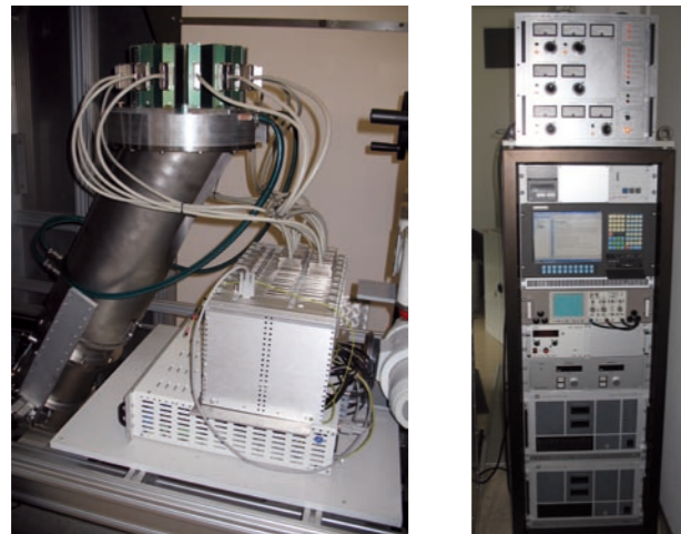
Fig. 3: Generator head with x-ray detector (left) and operating console (right) of the new electron beam tomograph.
