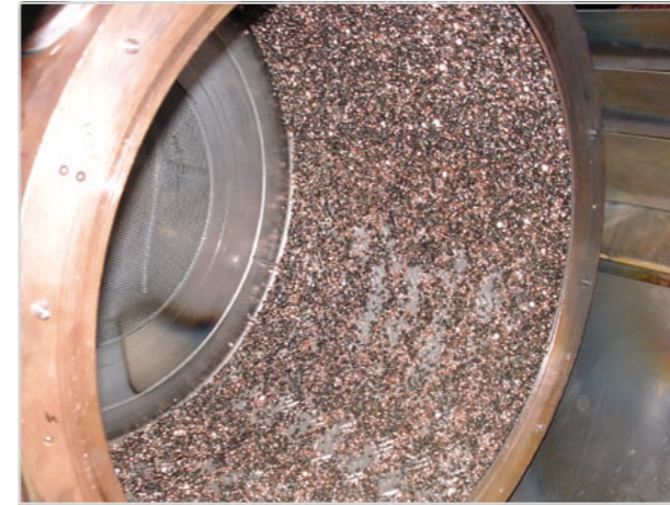
Fig. 2: Distribution of a charge of copper and steel rivets in a rotating drum. There is good mixing of the charge even after just one start-up.
