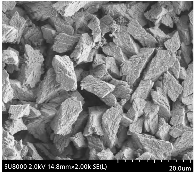
SEM image of the crystalline structure of biogenic limestone (CaCO 3 )
