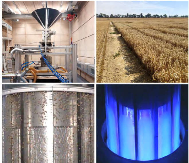
Novel cylindrical electron source for cost-effective seed treatment on test rig in high-voltage laboratory of Fraunhofer FEP
