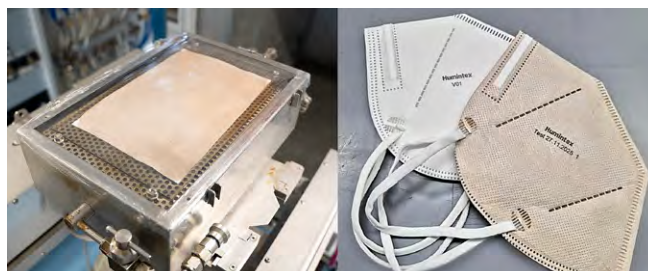
PLA nonwoven fabric with applied humic substances for the electron beam-assisted grafting process (left) and comparison of two FFP2 PLA respirator masks – one unmodified and one functionalized with humic substances (right)
