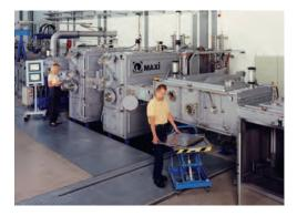
In-line vacuum coating equipment for sheets and metal strips MAXI
