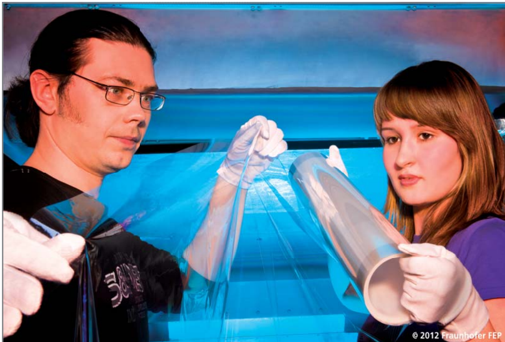
Fraunhofer researchers with an anti-reflective polymer film produced via plasma-etching. | © Fraunhofer FEP
