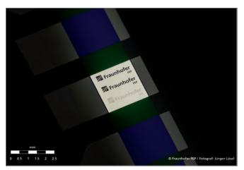
OLED patterned with an electron beam (Patterning: A. Rudzinski, Raith GmbH) © Fraunhofer FEP / Photographer: Jürgen Lösel Picture in printable resolution:www.fep.fraunhofer.de/press
