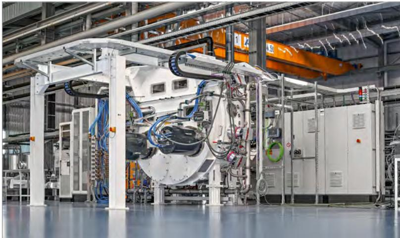
**VON ARDENNE FOSA LabX 330 Glass - coating system for flexible glass**
