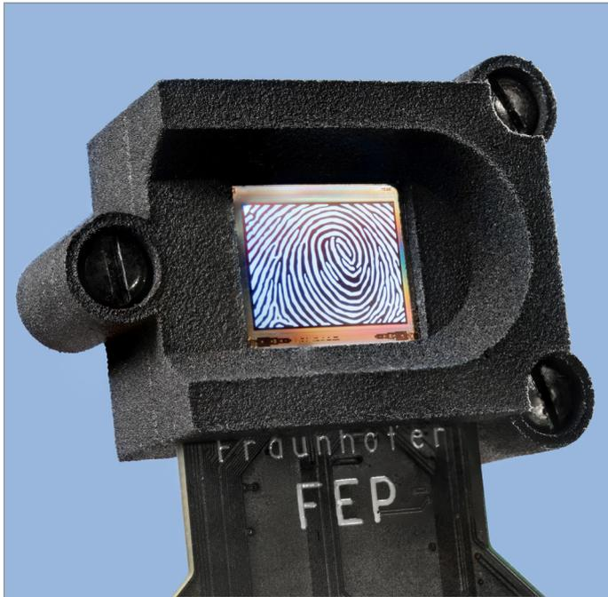
**High-resolution OLED-on-silicon fingerprint sensor**
