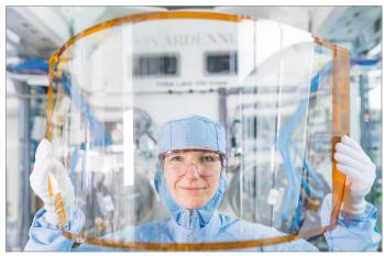
Ultra-thin flexible Corning® Willow® Glass with a glass thickness of 100  $\mu m$
