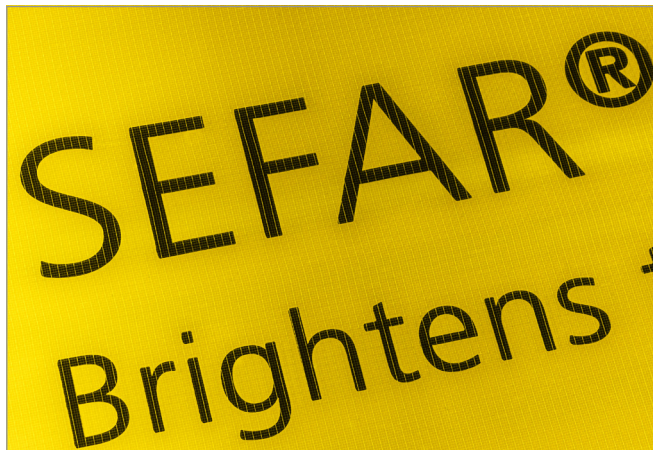
Roll-to-roll processed OLED on SEFAR TCS Planar substrates
