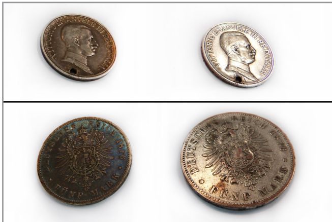
Coins before and after plasma treatment at Fraunhofer FEP
