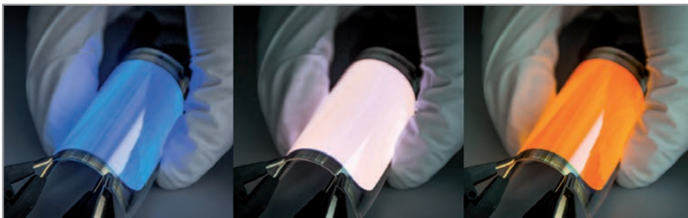
Adjustable-color OLED on flexible substrates
