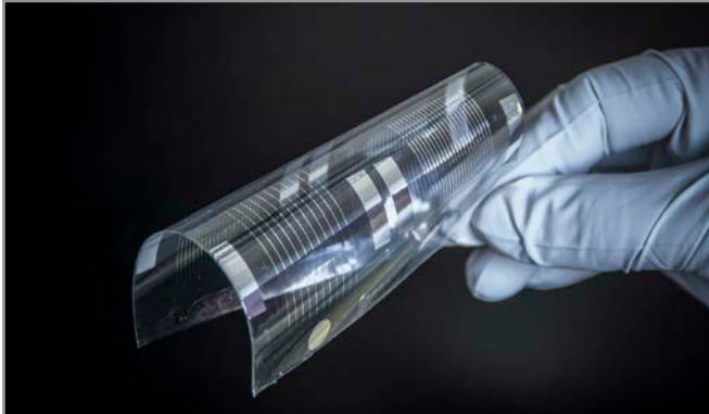
Biodegradable conductor structures on biodegradable polymer film
