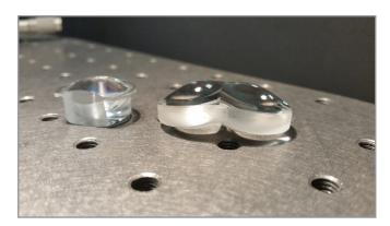
Thineyes® optical train for the LOMID project. On the left is an aspheric doublet lens and on the right a freeform lens. The LOMID optical architecture uses 2 aspheric and one freeform lens per eye, in order to seamlessly combine two high resolution microdisplays per eye. © LOMID project
