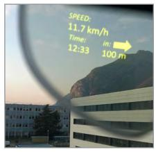
Incorporation of the ultra-low-power displays in data glasses © MICROOLED
