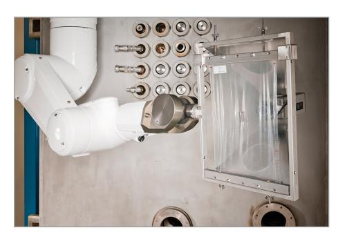
Sterilization of an implant screw using electron beam technology and 3D handling © Fraunhofer FEP Picture in printable resolution: www.fep.fraunhofer.de/press
