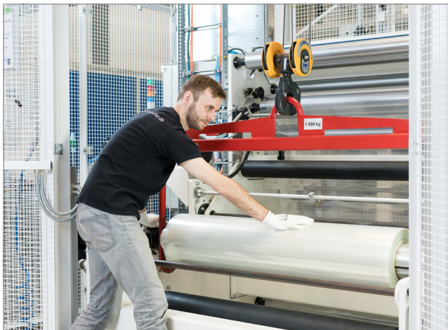
Flexible film substrate of 1.25 meter width at the roll-to-roll coating line „atmoFlex 1250“
