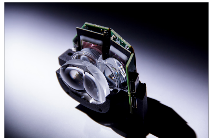
Optics of VR glasses with 2 large-area OLED microdisplays
