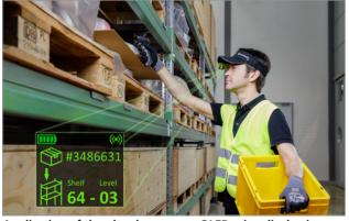
Application of the ultra-low-power OLED microdisplay in stock management © Fraunhofer FEP, photographer Claudia Jacquemin Picture in printable resolution: www.fep.fraunhofer.de/press
