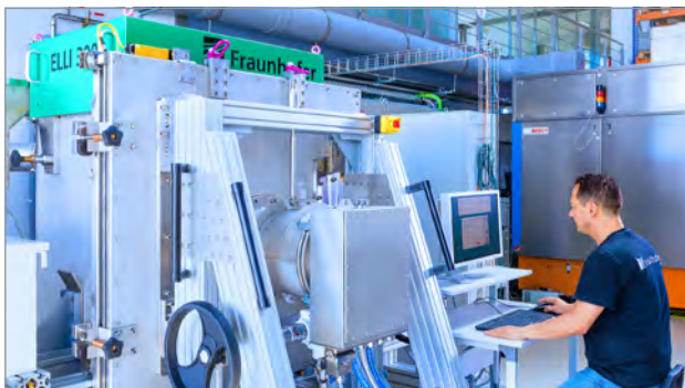
ELLI 300 – An innovative design for electron-beam treatment of liquids
