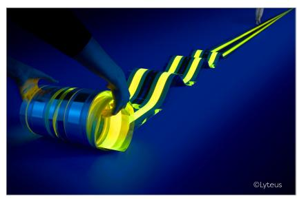
**15-meter roll-to-roll device is world's longest OLED** © Lyteus Picture in printable resolution: www.fep.fraunhofer.de/press
