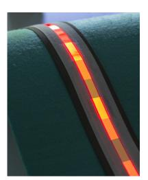
OLED luminous strips enable luminous surfaces with segmented control.
