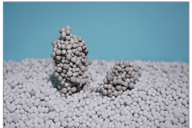
Aluminum coated granulate, as bulk material and sintered
