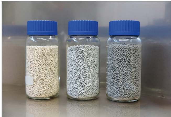
Zeolite granulate in original condition (left) and coated with aluminum (center, right)
