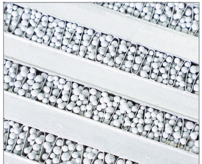
Fig. 3: Heat exchanger filled with aluminum coated zeolite pellets
