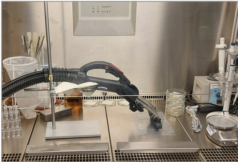
Test setup with steam vacuum cleaner for analyzing the disinfection success
