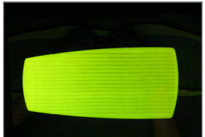
Illuminated OLED with a luminous area of 206 mm in length and 70 mm or 95 mm in width
