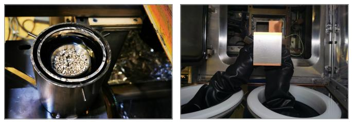
Lithium in its initial form as granulate and deposited as a thin film as the basis for manufacturing innovative and efficient next-generation batteries
