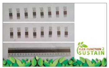
World's first organic photovoltaic cell on a film made of recycled polypropylene from drink pouch packaging material
