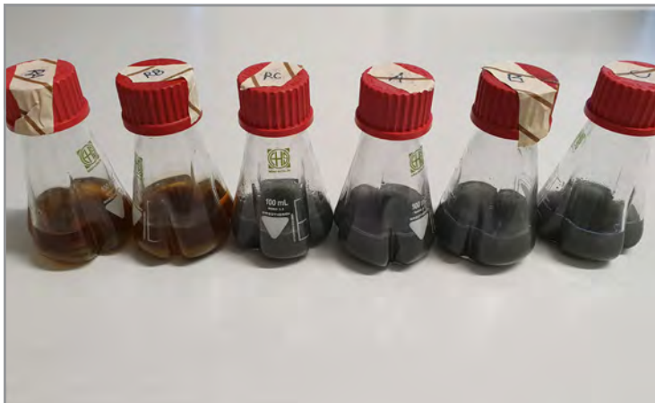
Samples with electron beam treated bacteria for bioleaching
