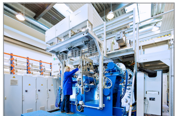
novoflex® 600 roll-to-roll pilot strip coater, on which the new process for the deposition of columnar silicon layers
