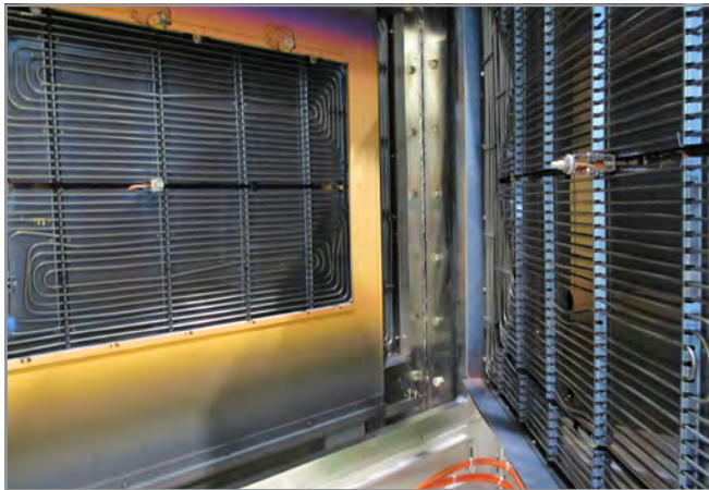
Newly developed measurement setup with sensor measuring head for in-situ characterization of coating processes at high process temperatures
