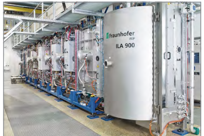
ILA 900 – Vertical in-line sputtering system for coating flat substrates, under clean room conditions with a magnetron length of 900 mm
