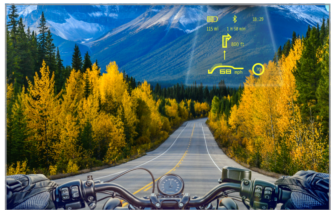
Already available and in use: The Head-Up Display for motorcycle helmets from "Tilsberk" (a brand of digades GmbH)
