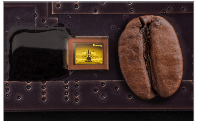
Size comparison of the new backplane with a coffee bean
